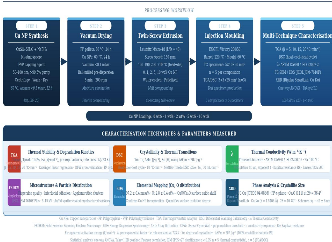
Figure 1. Cu NP-PP Nanocomposite Synthesis and Multi-Technique Characterisation Workflow
