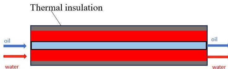
Figure 1. Schematic diagram of a heat exchanger of direct flow type (parallel flow)
