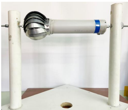
Figure 3. Experimental layout of a cylindrical blade with a metal active deflector (made of aluminum)
