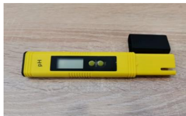
Figure 2. Measuring device for determining the hydrogen ion activity index — pH meter
