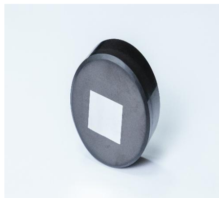
(b) surface after grinding and polishing
