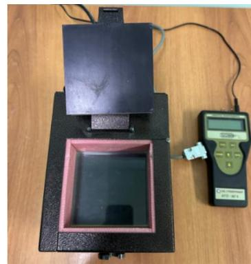
Figure 4. Heat conductivity meter ITP-MG4 100
