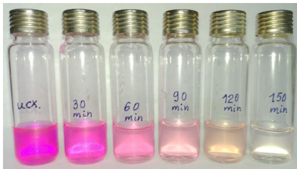
Figure 6. Photo of the RhB solution in the presence of the ZGP 7 sample subjected to UV illumination
