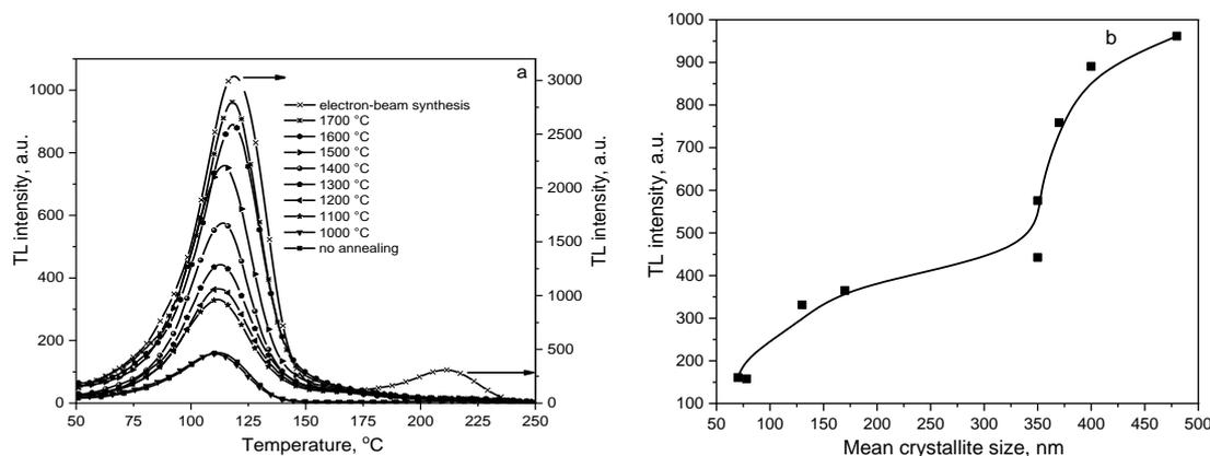
Figure 3. TL curves of  $ZrO_2$  ceramics synthesized under different conditions, after exposure to a test dose of a pulsed electron beam (15 kGy) (a) and dependence of TL peak intensity at 120 °C on the crystallite size (b)
