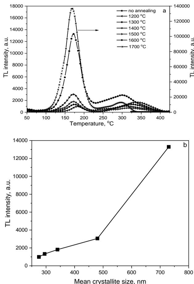
Figure 2. TL curves of  $\alpha-Al_2O_3$  ceramics annealed at different temperatures and exposed to a pulsed electron beam with 15 kGy dose (a) and dependence of TL peak intensity at 170 °C on the crystallite size (b)
