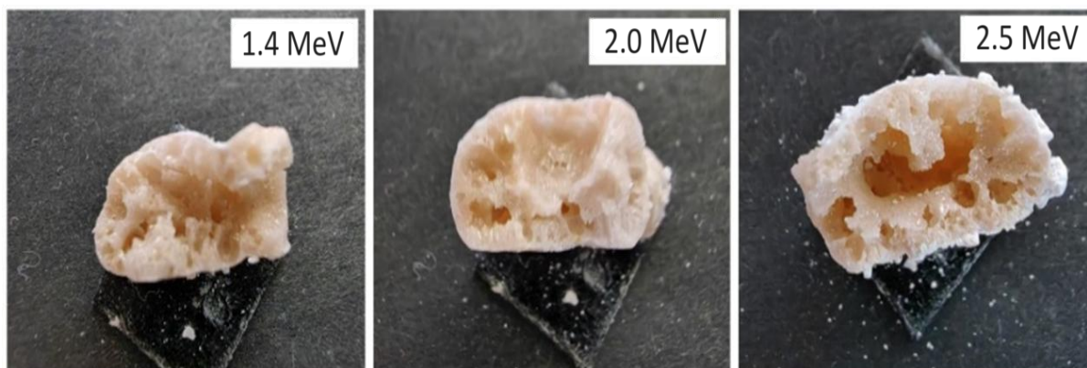
Figure 2. Optical images of transverse cleavages of droplets of synthesized HEC ( Y_{0.2}Yb_{0.2}Lu_{0.2}Eu_{0.2}Er_{0.2})_3Al_5O_{12} ) at different values of accelerating voltage
