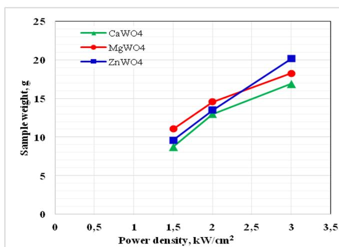
Figure 5. Weight dependence of CaWO<sub>4</sub>, MgWO<sub>4</sub>, ZnWO<sub>4</sub> tungsten ceramics on electron flux power density
