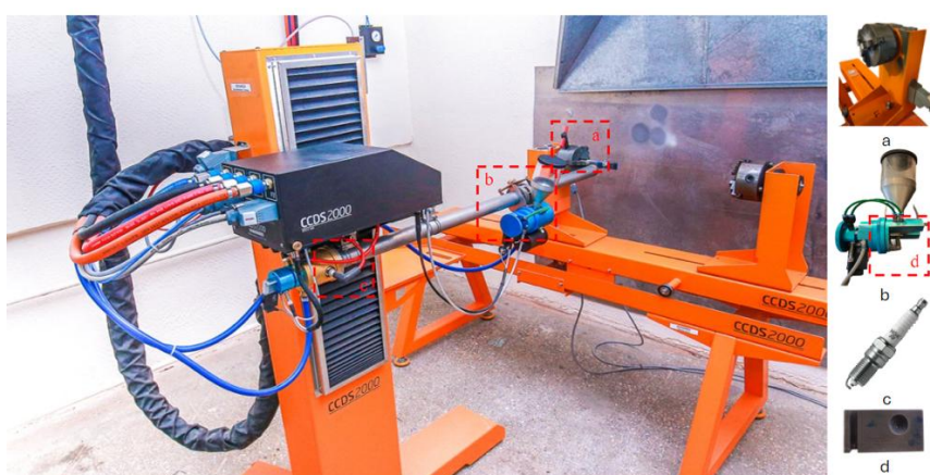
a — manipulator; b — powder dispenser; c — spark plug; d — dispensing plate
