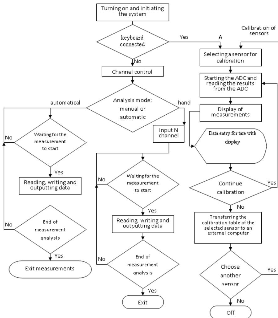
Figure 11. Algorithm of operation of the electronic unit SPU
