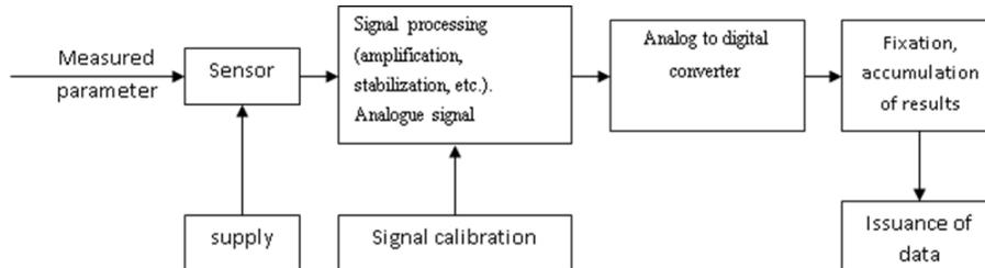
Figure 10. SPU channel structure
