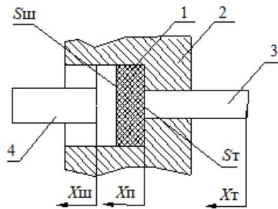
Figure 3. Scheme of the studied tracking device:  $X_T, X_{II}, X_{III}$  — displacement of the pusher, piston and rod, respectively;  $S_T, S_{III}$  are the areas of reactive washer 1 interacting with the pusher and rod, respectively
