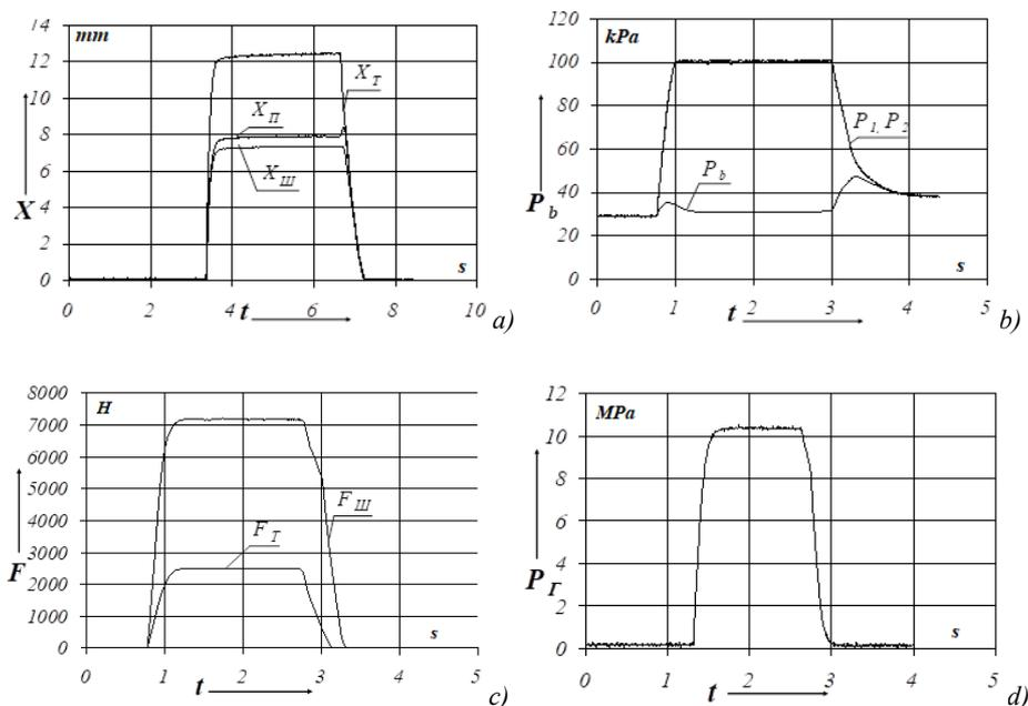
a) displacement  $X = f(t)$ ; b) rarefaction  $P_b = f(t)$ ; c) efforts  $F = f(t)$ ; d) pressure in the load drive  $RG = f(t)$ ;  $X_I, X_{II}, X_{III}$  — displacement of the pusher, piston and rod, respectively;  $P_b, P_1, P_2$  — change in pressure in the vacuum cavity and atmospheric cavities;  $F_I, F_{III}$  — force on the pusher and rod, respectively
