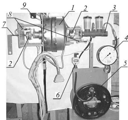
1 — vacuum brake booster under research; 2 — force sensors; 3 — the main brake cylinder; 4 — manometer;
