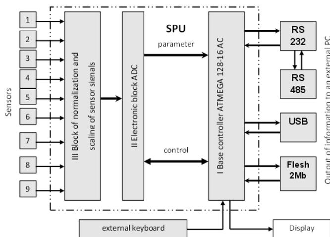
Figure 12. Block diagram of the measuring complex
