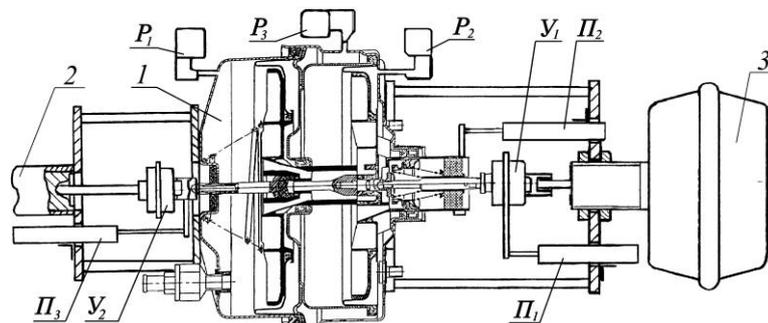
1 — vacuum booster under research; 2 — load; 3 — pneumatic chamber;
