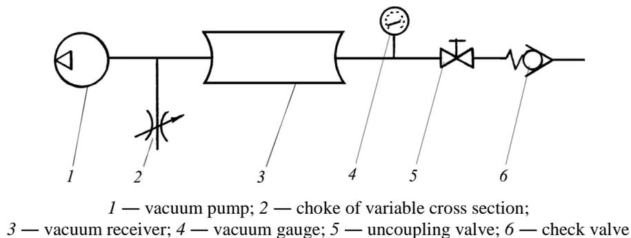
Figure 5. Diagram of the vacuum drive
