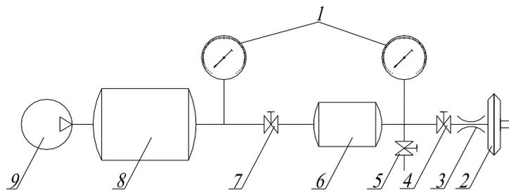
1 — pressure gauges; 2 — pneumatic chamber type 9; 3 — throttle; 4 — valve for flowing the receiver into the pneumatic chamber; 5 — valve for setting the pressure in the receiver; 6 — working receiver; 7 — valve for filling receiver 6; 8 — storage tank; 9 — stationary compressor
