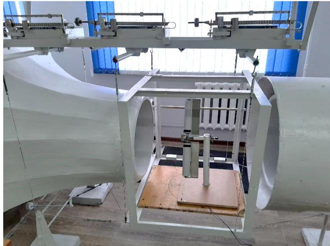
Figure 1. An experimental sample of a two-bladed layout
