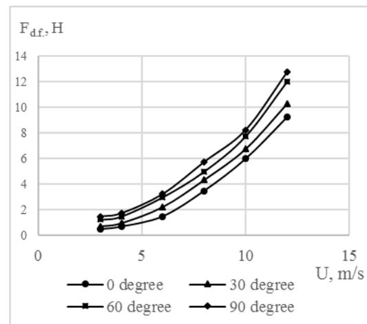
Figure 5. Graph of the dependences of the drag forces of the sail blades on the flow velocity at different angles  $\gamma$  of the apex of the triangular blade
