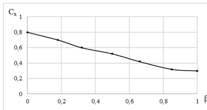
Figure 6. Dependence of the aerodynamic coefficient (drag) from  $\beta$
