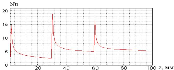
Figure 4. Nusselt criterion change along the pipe length
