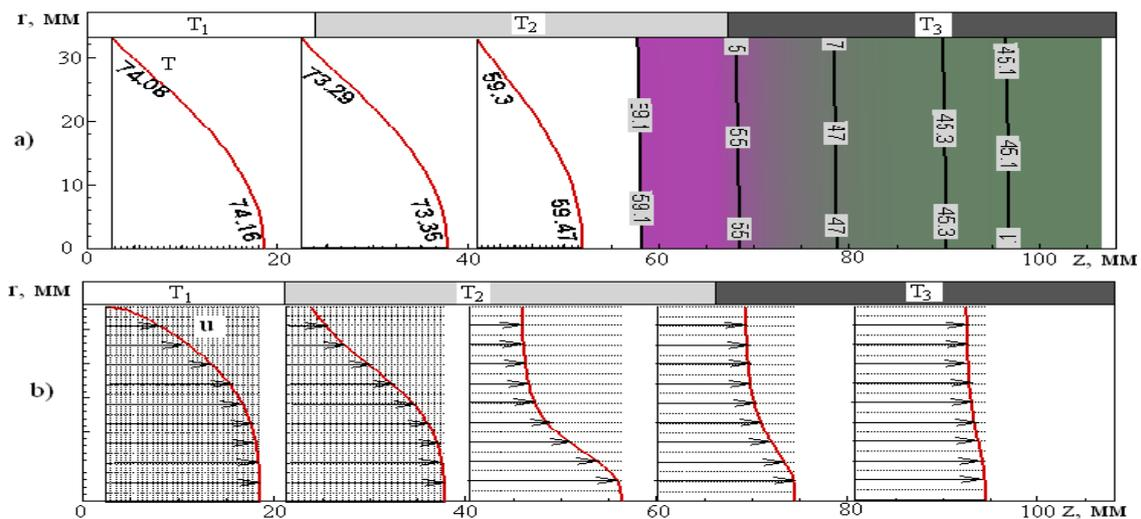
Figure 3. Temperature (a) and speed distribution (b) along the pipe length:
