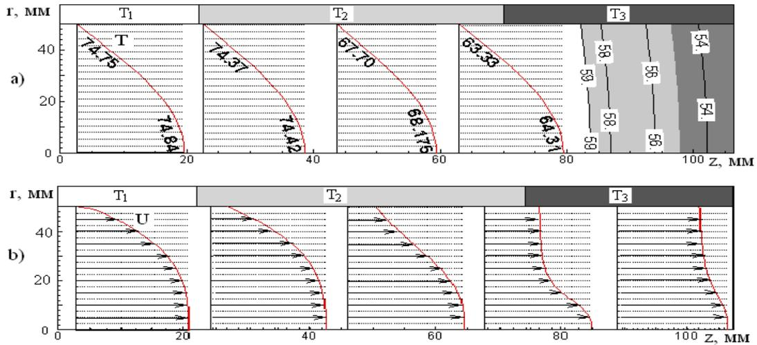
Figure 2. Temperature (a) and speed distribution (b) along the pipe length:
