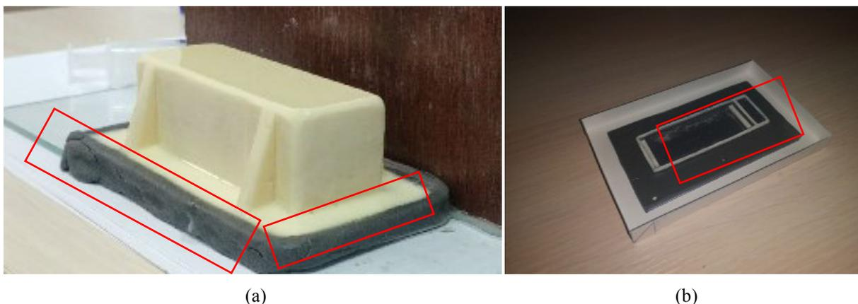
Figure 6. Refinement of the printed model: a — refilling the plastic on the edges of the upper body, b — increasing the height of the bottom body rim with paper
