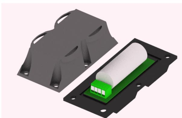
Figure 2. The 3D model of building a square enclosure around the board
