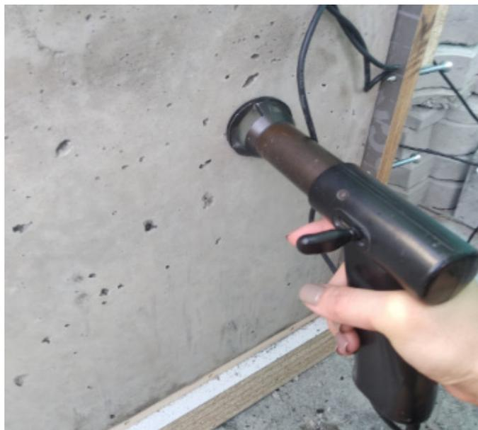
Figure 10. The strength tests by IPS MG4
