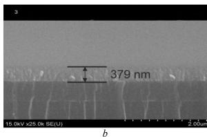
Figure 1. SEM-images of chip  $\alpha$ -C (a) and  $\alpha$ -C<sub>53.3</sub>:B<sub>43.2</sub> (b) of CC
