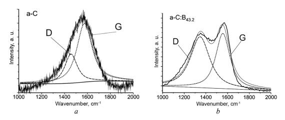
Figure 3. Raman-spectra  $\alpha$ -C (a) and  $\alpha$ -C<sub>53.3</sub>:B<sub>43</sub> (b) of CC
