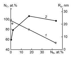
Figure 2. Dependancy diagram of carbon component  $N_C$  content (1) and grain  $R_g$  average size (2) in CC structure on  $N_B$  concentration of dopant boron atoms.
