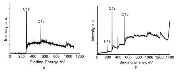
Figure 4. XPS  $\alpha$ -C (a) and  $\alpha$ -C:B<sub>43 2</sub> (b) CC
