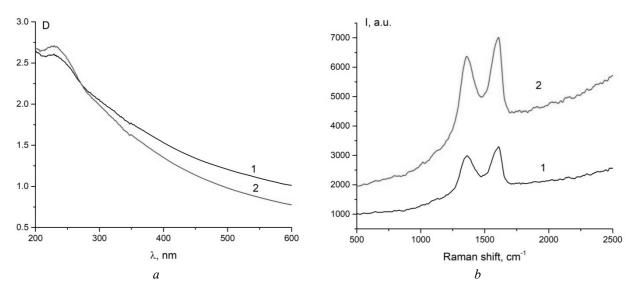
Figure 2. Absorption (a) and Raman (b) spectra of GO dispersion before (1) and after (2) ablation
