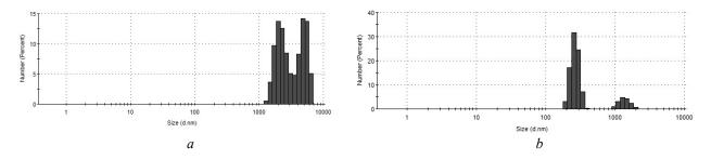
Figure 1. Size distribution of GO particles in water before (a) and after (b) laser irradiation
