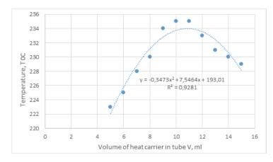
Figure 4. A plot of temperature change versus coolant volume from 5 to 15 ml
