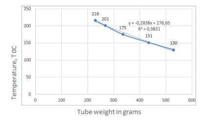
Figure 5. Dependence of the surface temperature of the case of an electrovacuum heater on its mass
