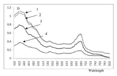
Figure 5. Absorption spectra of solutions of a green leaf at different concentration of chlorophyll. Increase of concentration of chlorophyll comes from a curve 3 to a curve 1
