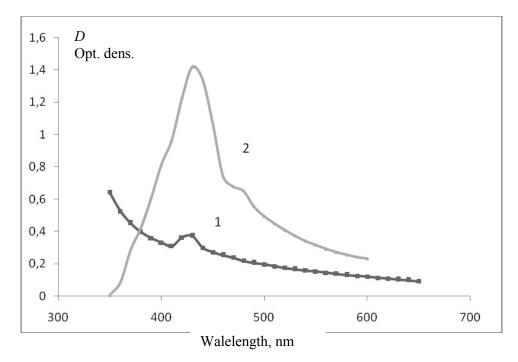
Figure 6. Absorption spectrum of nanoparticles of silver: after repeated disolution (1), in initial solution before introduction of particles of silver (2)
