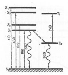
Figure 3. Scheme of singlet and triplet energy levels of a molecule of a chlorophyll and direct pieces correspond to absorption, wavy shooters — blooms. Figures specify a wavelength in nanometers
